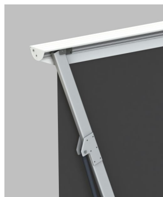
Rear cross-profile system with gas springs for perfect tensioning of the screen surface
